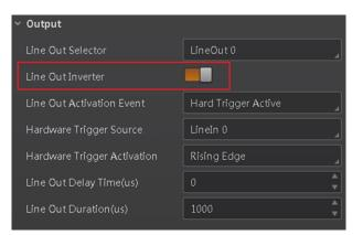
Figure 7-25 Enable Line Out Inverter
