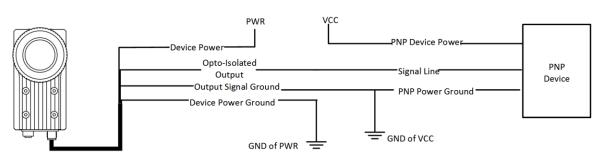
Figure 3-6 Output Signal Connecting to PNP Device
