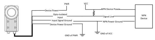
Figure 3-5 Input Signal Connecting to NPN Device with Pull-Up Resistor
