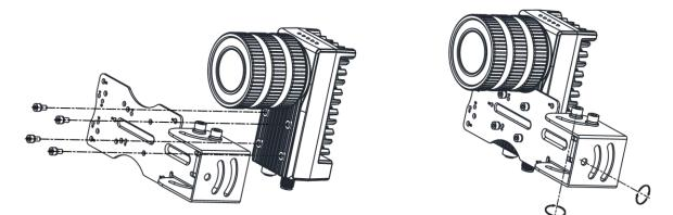
Figure 4-3 Side Installation
