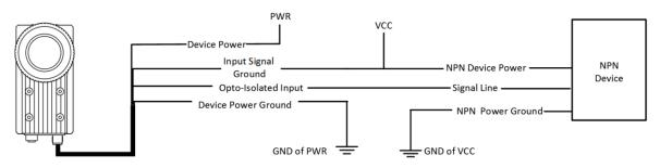
Figure 3-4 Input Signal Connecting to NPN Device without Pull-Up Resistor
