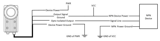
Figure 3-7 Output Signal Connecting to NPN Device without Pull-Up Resistor
