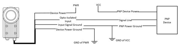
Figure 3-3 Input Signal Connecting to PNP Device
