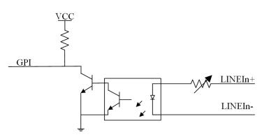
Figure 3-1 Internal Circuit of Input Signal
