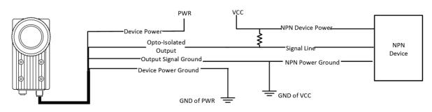
Figure 3-8 Output Signal Connecting to NPN Device with Pull-Up Resistor
